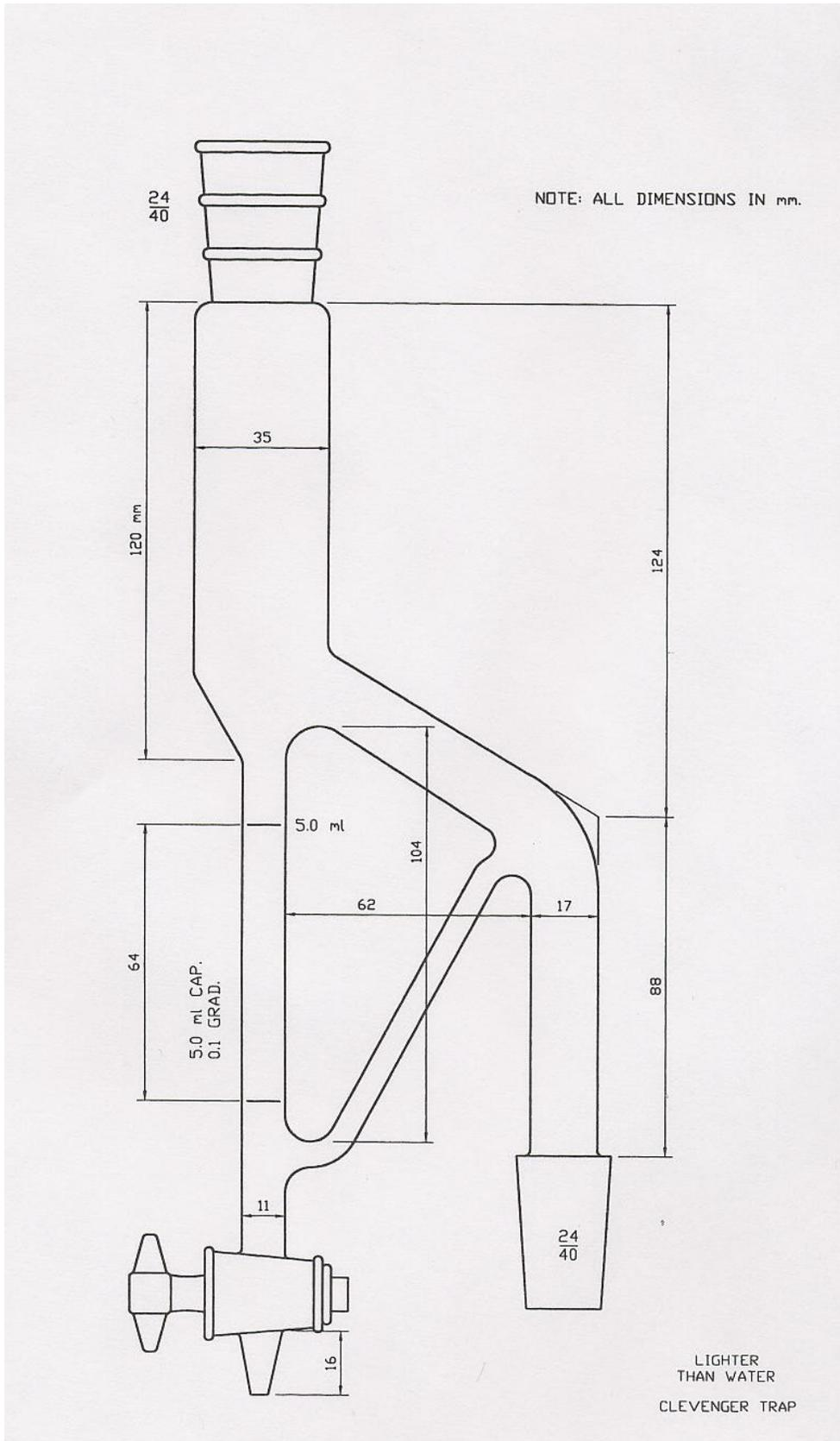
Figure 1b. Lighter than water Clevenger trap.
