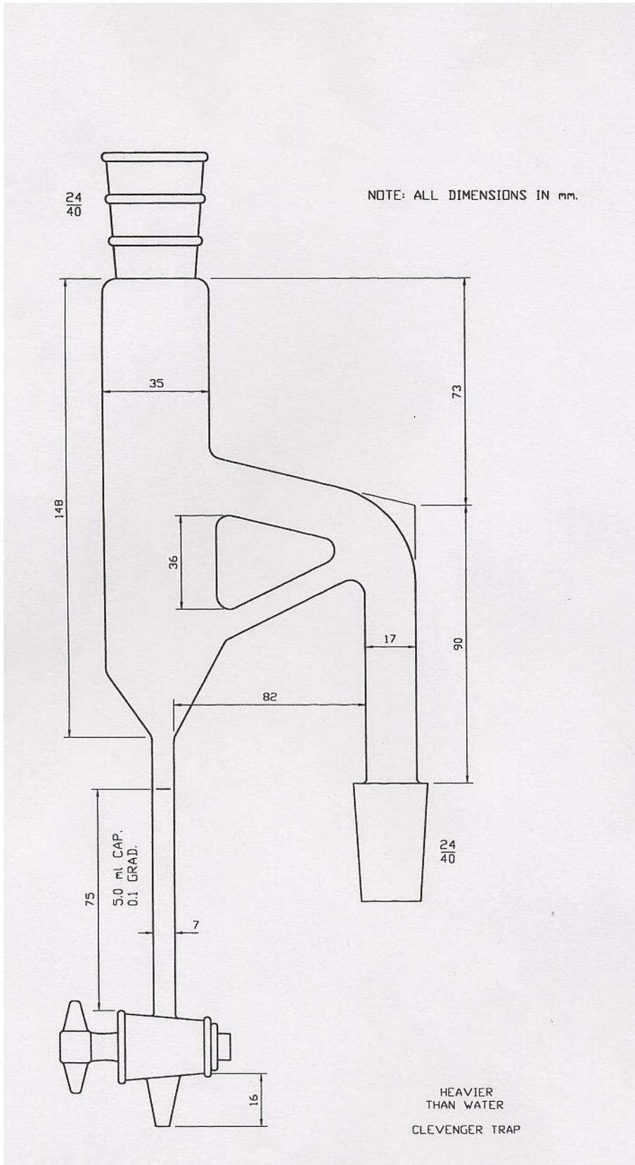
Figure 1a. Heavier than water Clevenger trap.
