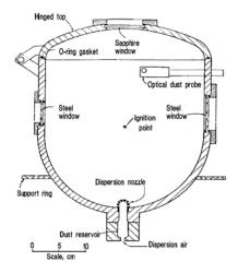
Figure 1: 20-Liter Explosibility Test Chamber
